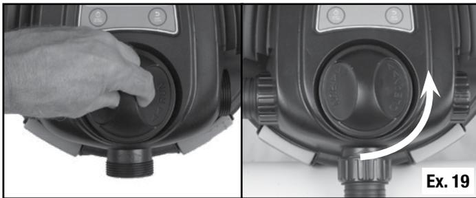
**NOTE:** The valve can be a little stiff to turn if it hasn't been moved in a while. Do not use tools which might crack the handle. The valve assembly can be removed from the lid for cleaning and lubrication with silicone grease. We recommend doing this if the valve becomes very stiff to turn.
